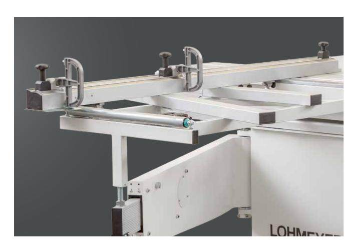
The double roller carriage accomodates the cross slide. A precise factory set up guarantees high accuracy of parallelism to the saw blade for many years.
