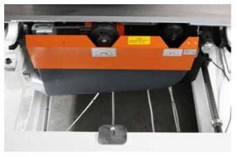
Besides the slide table, the saw aggregate is another main element of the sliding table saw.
